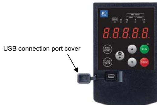
Connect the inverter directly to a PC with the USB cable. FRENIC Loader allows the user to edit, check, and manage inverter function codes, and perform remote operations such as monitoring data while the inverter is running, and starting and stopping the inverter. The running status and alarms, etc. can also be monitored.
